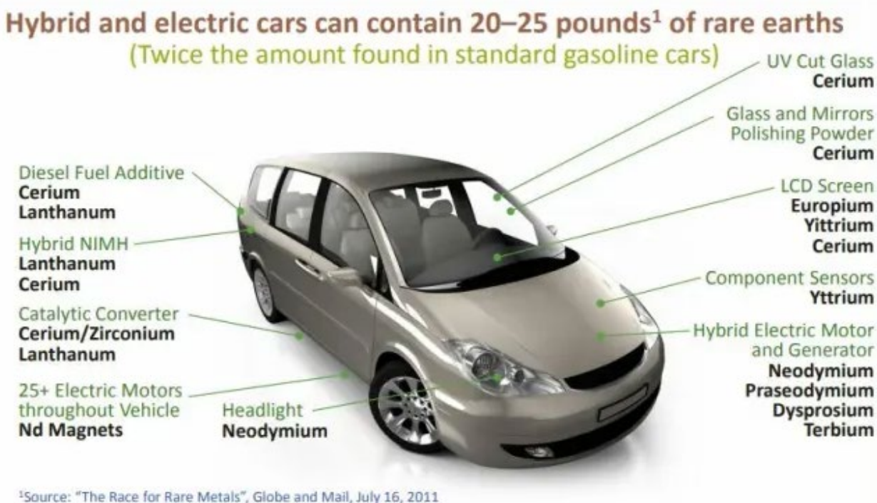
Figure 4: Amount of Rare Earths Required in the Manufacture of an Electric Vehicle
